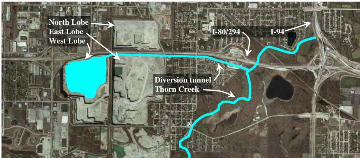
High flows from Thorn Creek flow through a diversion inlet structure, drop 230 feet down a 24-foot diameter shaft, and flow through an 8,000-foot long, 22-foot diameter diversion tunnel into the west lobe reservoir.
